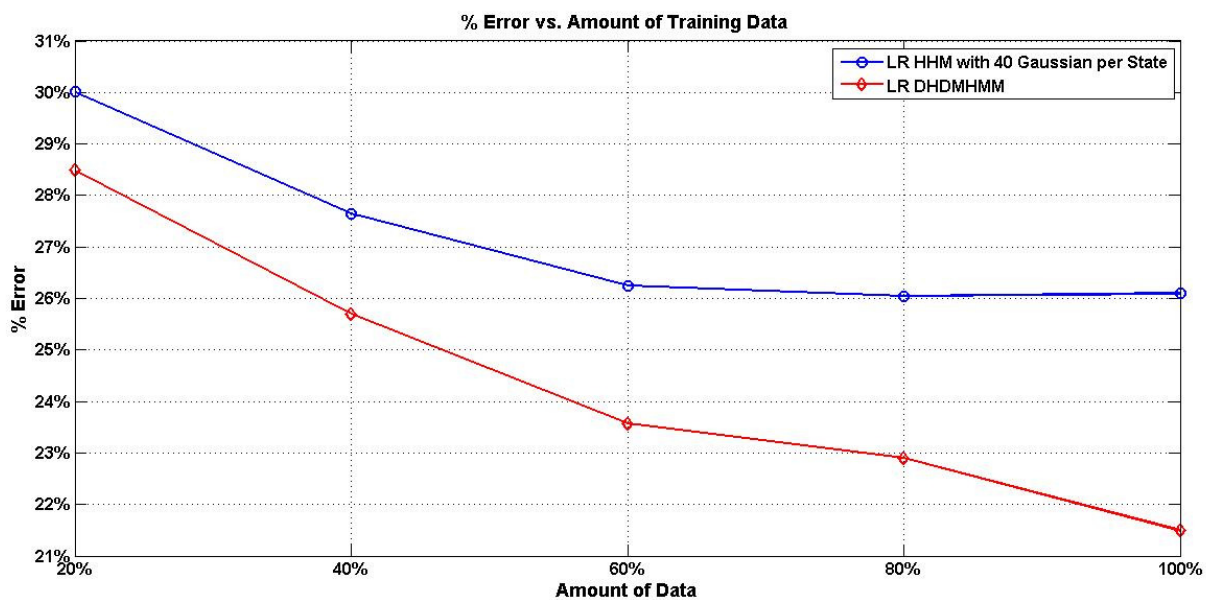
Fig. 7. Error rate vs. amount of training data for LR DHDHMM and LR HMM
