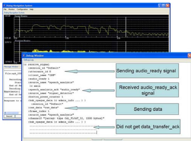
Figure 6: A debug window showing an audio data transfer error
