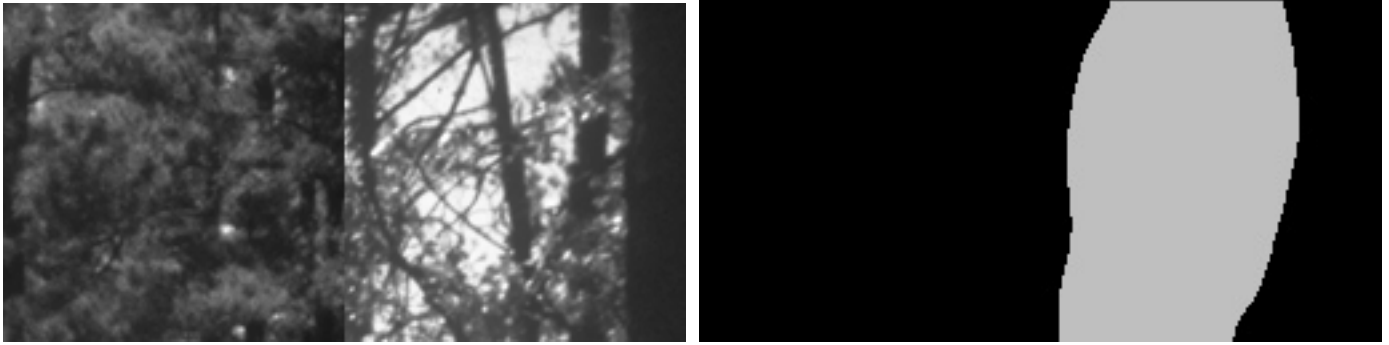
Figure 9. The image consists of two forestry regions. The left half is a typical “foliage” block, and the right half is a “bgsky” block. In the segmentation image, the black region stands for hypotheses for the “foliage” category, while the grey color is used for “bgsky”. The pixel classification error rate was 19.6%
