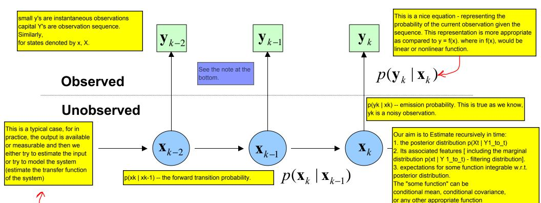
Filtering is the problem of sequentially estimating the states (parameters or hidden variables) of a system as a set of observations become available on-line.
