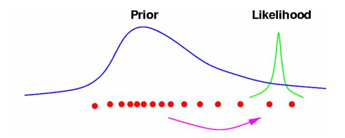
Use Gaussian approximation (i.e. Kalman filter) to generate proposal by combining new observation with prior
