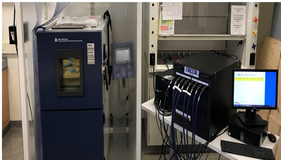
Figure 6.1. Maccor model 4200 and thermal chamber.
