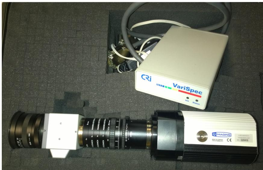
Figure 5.4: Hyperspectral camera acquisition system (Retiga EXi F-M-12-C)
