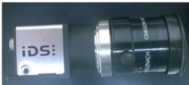
Figure 5.5: TIP camera (IDS UI-3240CP-NIR) and lens
