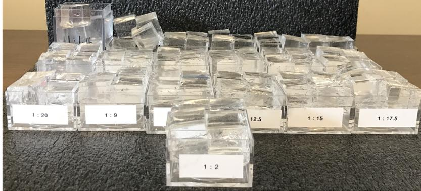
Figure 4.3: PDMS samples from Instron test
