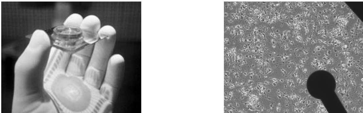
Fig. 2: Substrate-integrated MEA dish. The microscopic image of the electrode (black) and neurons
