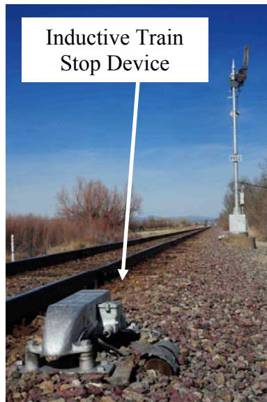
Figure 12, An inductive Train Stop
