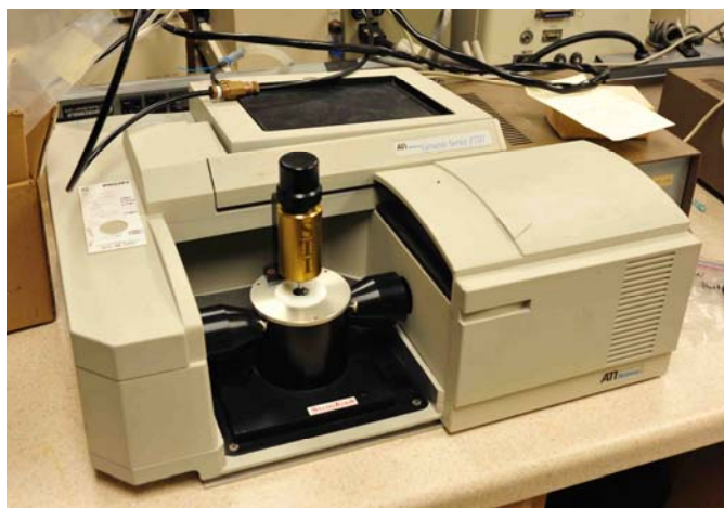
Figure 33, The laboratory FTIR set up to examine top of rail contaminants
