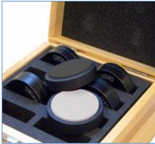
Figure 12: The Spectralon reflectance standards SRS-99 and SRS-02.
