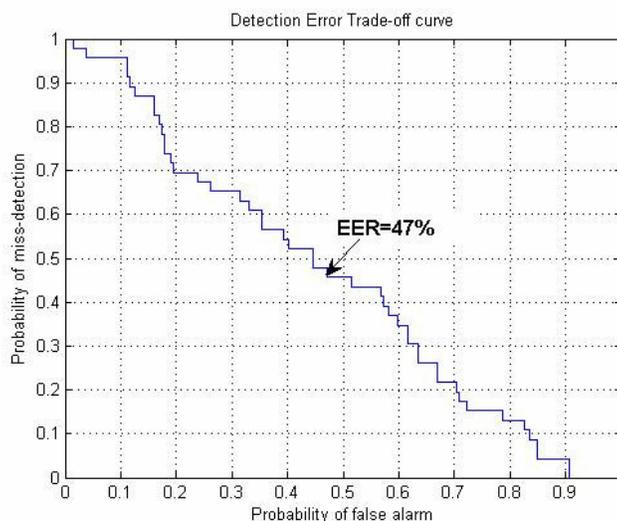
Figure 9 Detection error trade-off curve for a speaker verification-based fatigue detection system
