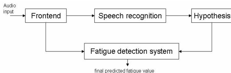
Figure 10 Integration of the fatigue detection system with an ASR system
