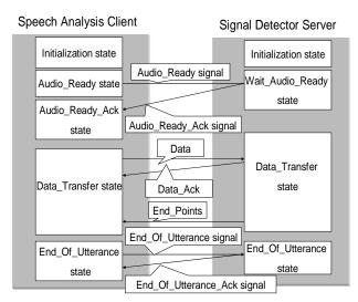
Figure 4. Handshaking between the Speech Analysis client and the Signal Detector server
