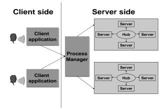
Figure 2. The Process Manager module controls multiple applications and servers.
