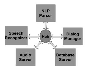
Figure 1. An overview of a DARPA Communicatorbased dialog system architecture.
