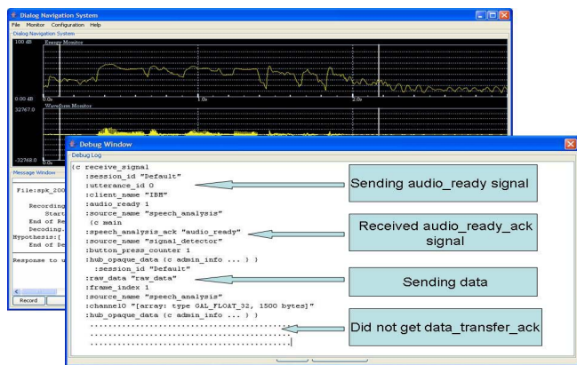
Fig. 6. A debug window showing an audio data transfer error
