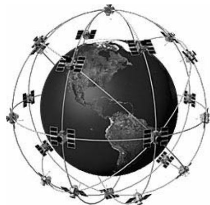
Figure 2. GPS consists of 24 satellites of which at least 5 can be seen from any point on the globe.
