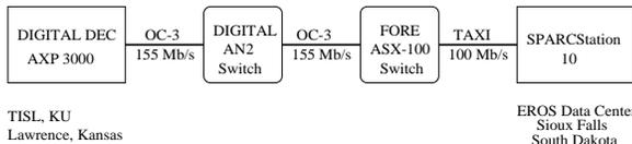
Figure 7. Experimental Set Up for TCP/ATM Performance under Rate Mismatch Conditions
