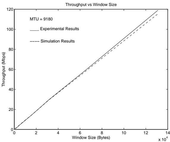
Figure 6. ATM WAN Performance vs TCP Window Size
