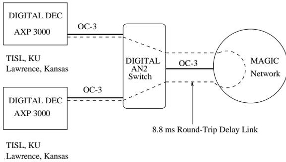
Figure 4. Experimental Set Up for ATM WAN Performance vs TCP Window Size
