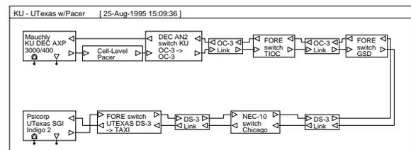
Figure 10. Simulation Model of a Single Connection in the AAI Network
