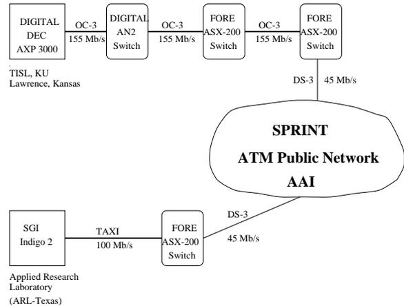
Figure 9. Experimental Set Up of a Single Connection in the AAI Network
