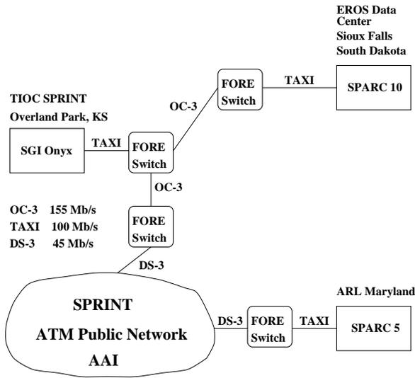
Figure 11. Experimental Set Up of Simultaneous connections over the AAI Network
