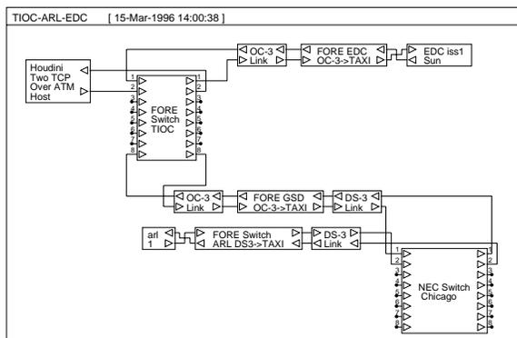
Figure 12. BONEs model of Simultaneous connections over the AAI Network
