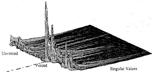
Figure 8: Singular Values of Speech Data with SNR = 30.7 dB
