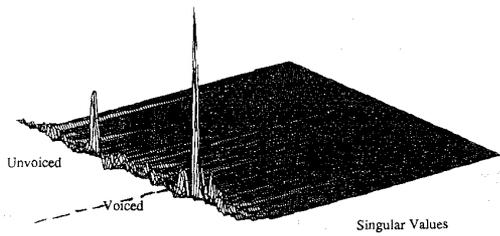
Figure 7: Singular Values of Speech Data with SNR = 18.2 dB
