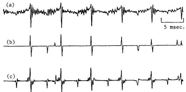
Figure 6. A Comparison Between the MPLPC and the ZMPLPC Excitations: (a) Original Residual (40 msec. Duration); (b) MPLPC Excitation; (c) ZMPLPC Excitation.
