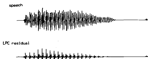
Figure 2. Example where the pitch period is easily found in the residual but not in the speech.
