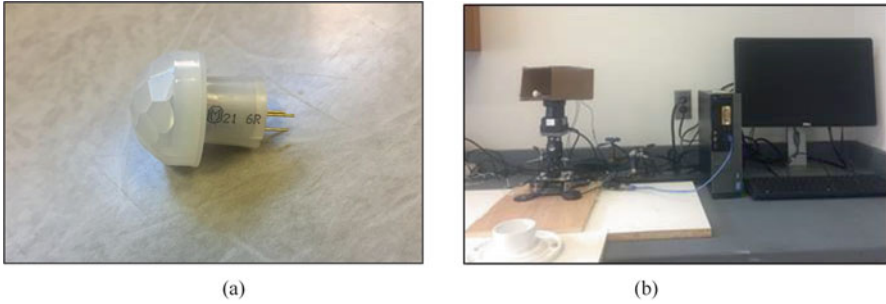
Fig. 1 Novel MI-PIR system including the (a) the Panasonic AMN24112 and (b) the full design
