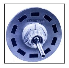
Part no. 8375 magnetic saw holder shows detail of 12" diameter backing plate inlaid with permanent magnets. Expanding center bushing tightens against the saw eye for a perfectly round saw. The entire holder turns freely on two ball bearings which fit over the standard 7/8" mandrel used on all Armstrong automatic circular saw sharpeners as well as the No. 84 Autopoint automatic swage and shaper
