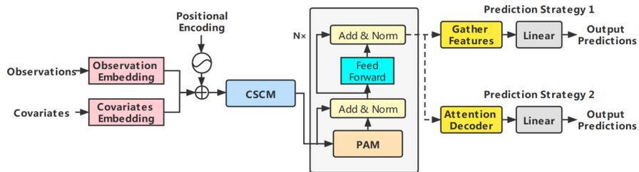
**Figure 14.** The architecture of Pyraformer
