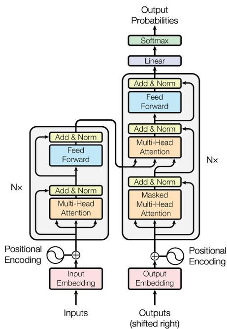
**Figure 4.** The original transformer model proposed in [148]
