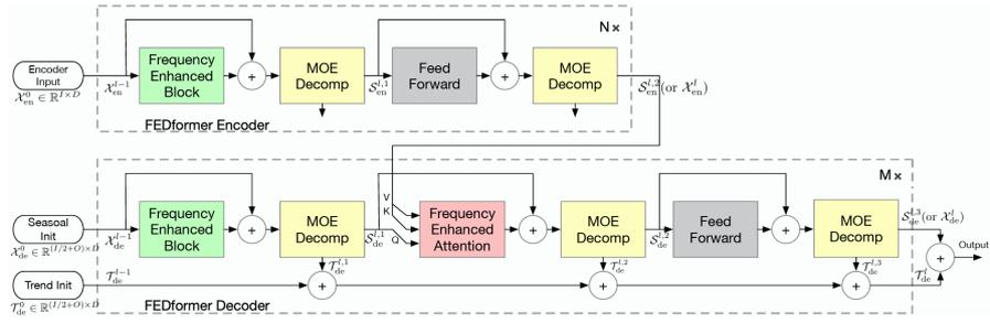
**Figure 16. Fedformer Structure**
