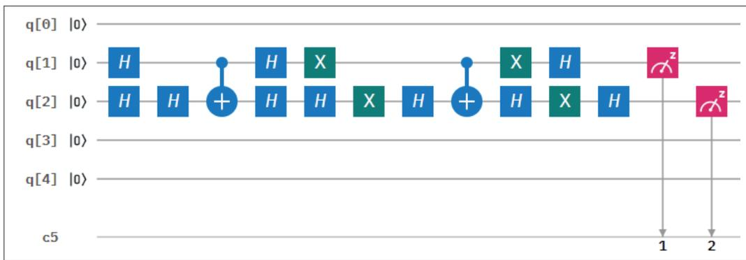
FIGURE 2. Grover's algorithm implementation using the circuit composer.
