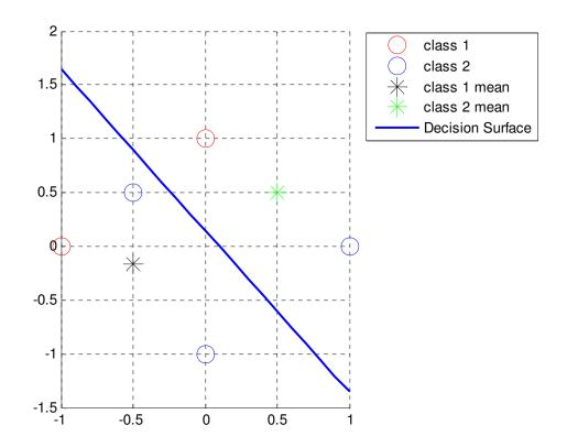
The new centers of the clusters have shifted as expected. A decision surface has been overlaid perpendicular to the line between the two cluster centers.
