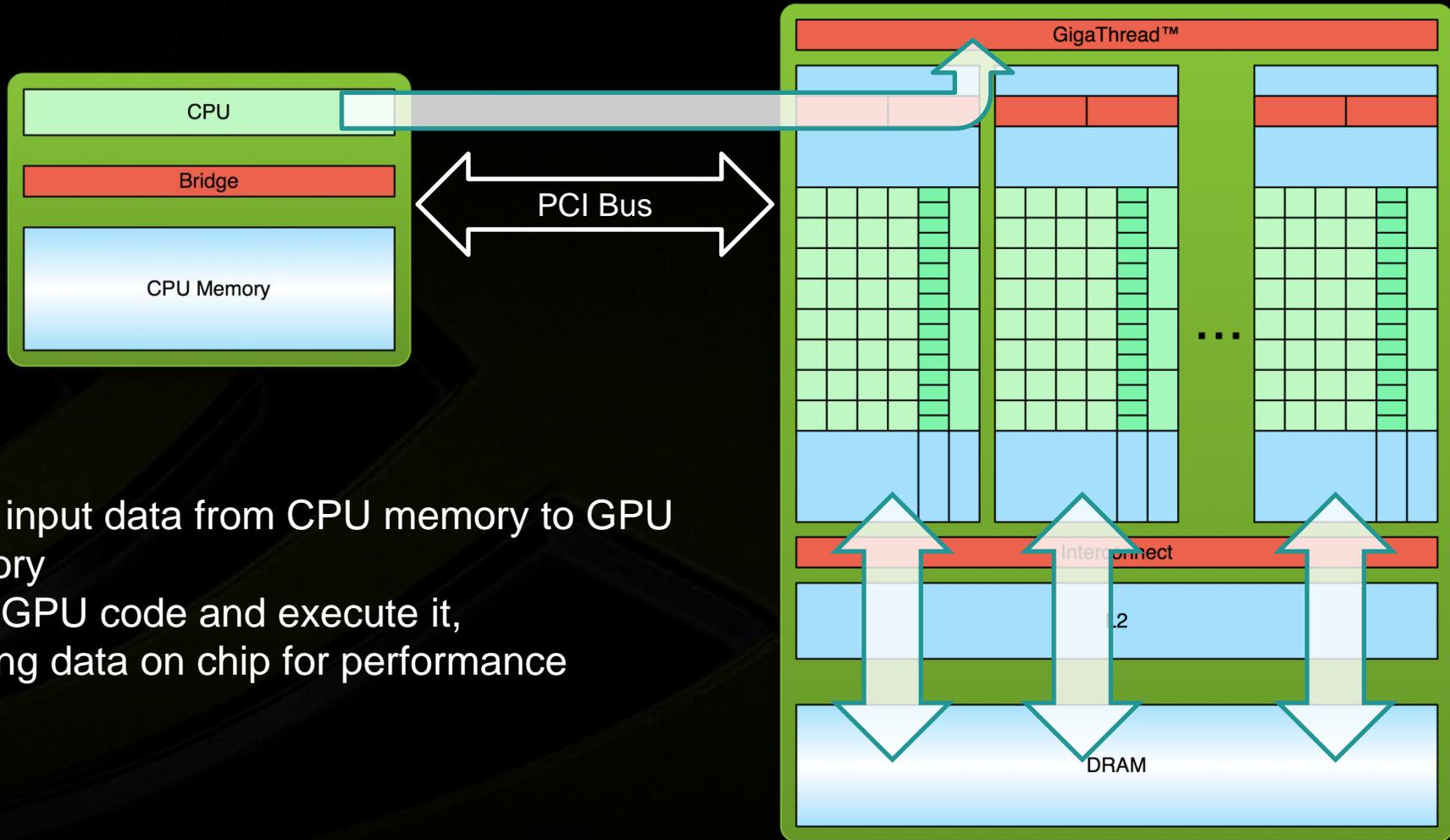
1. Copy input data from CPU memory to GPU memory
