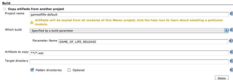
Figure 12.6. Specify where to find the artifacts to be deployed
