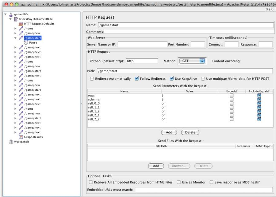
Figure 6.24. Preparing a performance test script in JMeter
