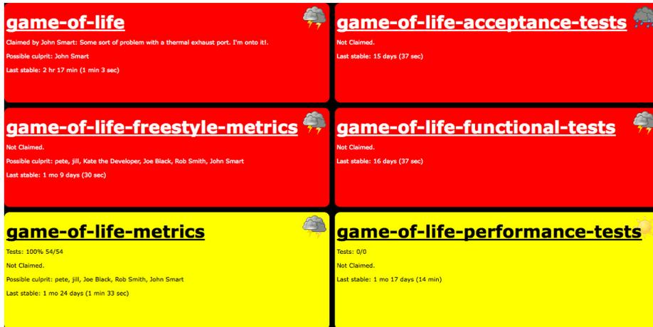
Figure 8.8. Displaying a build radiator view
