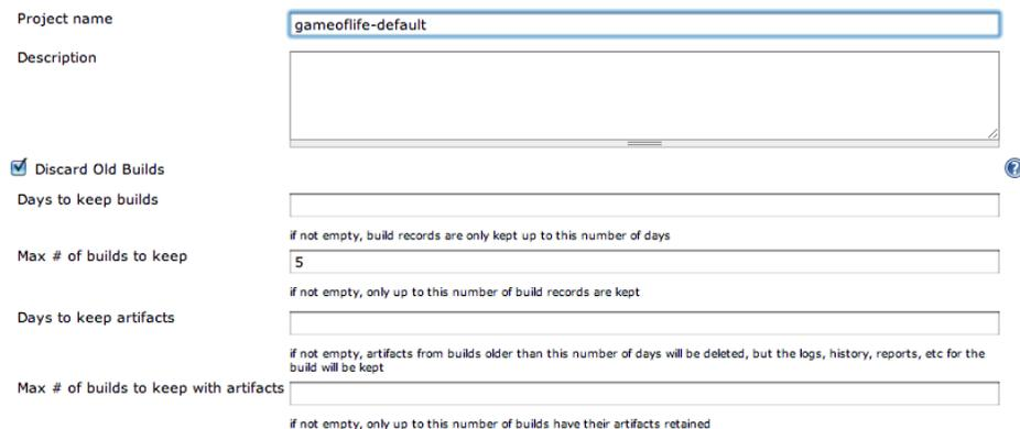
The screenshot shows the Jenkins project configuration page for a project named "gameoflife-default". The "Discard Old Builds" checkbox is checked. Below it, there are four input fields for configuring build retention:
