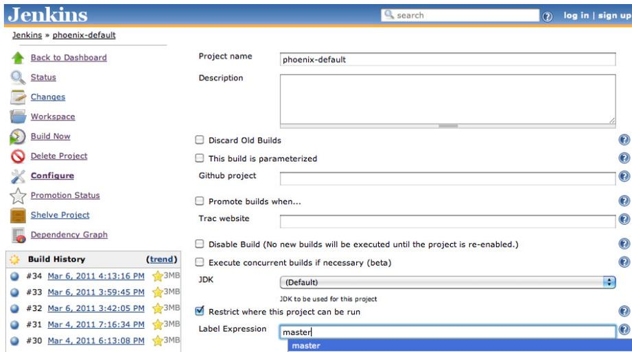
Figure 11.15. Running a build job on a particular slave node
