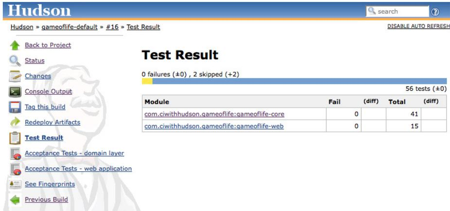
Figure 6.10. Jenkins displays skipped tests as yellow
