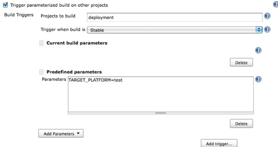
Figure 10.18. Passing a predefined parameter to a parameterized build job
