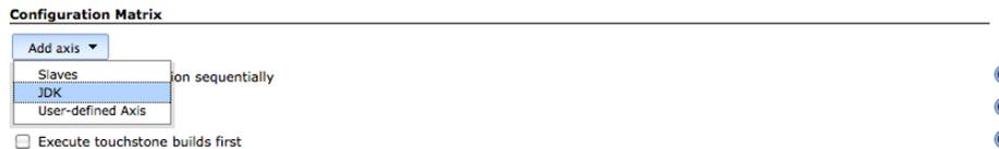
Figure 10.20. Adding an axis to a multiconfiguration build
