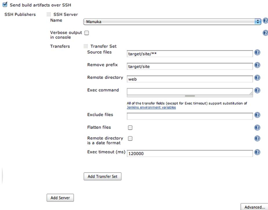
Figure 12.15. Deploying files to a remote host in the post-build actions
