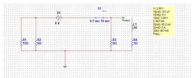
This is the Multisim circuit diagram, the probe shows steady state (before the switch is flipped), and shows 2V and .667 mA. This verifies our steady state analysis of the circuit, but it does not show the whole picture. To see the entirety of the circuit's transient response, we need to use Multisim to do a transient analysis. The result of this analysis can be seen below.
