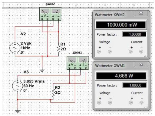
From this Multisim, we can clearly see that 1 Watt is dissipated in the 2Volt peak signal, whereas 4.66 Watts are shown in the signal from 3a.
