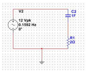
We can choose a 1 Farad capacitor to replace the -j1 capacitor in the problem because we have set the frequency to 1 / 2pi. This makes the capacitor's impedance  $\frac{1}{(\frac{2*pi}{2*pi}*C*j)}$ . Meaning a 1 farad
