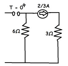
From this, we can infer the time constant of L/R is equal to 2 H / 9 Ohms. We also know the form of the solution is  $C1 + C2e^{-9t/2}$ . From this circuit, we can get the equation of  $C1 + C2 = I_L = 2/3A$ . By looking at the circuit at  $T = \infty$  we can get the second equation to find our constants. At  $T = \infty$ , Our inductor is a short once again, and since it is cut off from any source the current through it must be zero. Therefore, C1 = 0, and the
