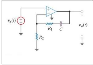
We have a working model of the ideal op-amp which we can use to solve this circuit to get its transfer function. We should first set the circuit in to the Laplace domain. Resistors stay the same and the
