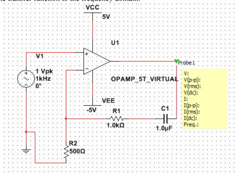
We know that the impedance of a capacitor as frequency increases becomes smaller and smaller, until the capacitor acts as a short. This gives us the final gain of  $1 + \frac{RI}{R2}$ , or in this case just 3. Since V<sub>in</sub> is just 1V, we expect our output to be 3V. Multisim verifies this:
