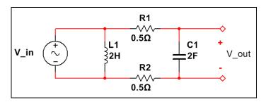
The first step to solving this problem is to convert the circuit to its Laplace domain equivalent. Also, since the branch which has the inductor and the branch which has the two resistors and the capacitor are in parallel, we can concern ourselves only with the second branch since they both have a voltage drop of V\_in. The new circuit can be shown as:
