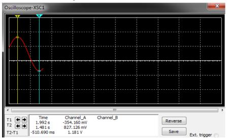
To get the average value of our sine wave and convert to Vrms, we can take the peak to peak voltage displayed (1.181V), and dividing by  $2\sqrt{2}$ . With this, we get our V<sub>o</sub> to equal approximately .41 Vrms, which is close to our initial idea of .4 Vrms. Multisim confirms all the calculations we have done.
