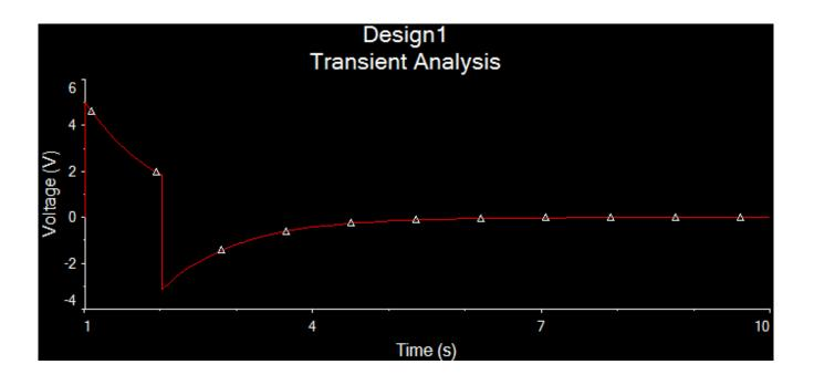
Doing a transient analysis gives us the above graph, which looks exactly like Matlab predicted it would. Thus, Matlab and Multisim corroborate with one another, and prove that the output voltage of the circuit should look like this.
