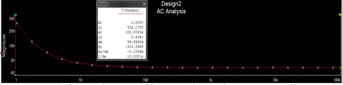
As you can see, the frequency increases, and the output voltage reaches an asymptote at 3V.
