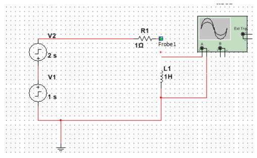
In Multisim 12.0, they introduced a step-function source, so it's simple to just put a source u(t-1), and a source in the opposite direction u(t-2) and check our results. We can do a transient analysis and check the graph of Vout over time.
