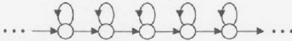
Figure 8(a). A simple progressive HMM topology. In general, the duration probability density function at a state has an exponential behavior.
