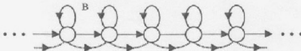
Figure 8(d). A fenonic baseform topology. The dashed line indicates a transition that produces no output.
