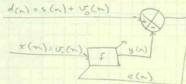
The filter,  $f$ , is adapted based on feedback from the system output  $e(n)$ .
