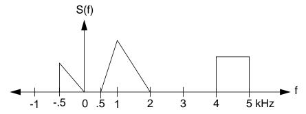
(a) Design a digital system that transmits this signal over the minimum possible bandwidth, and minimizes the computational and memory requirements. Be as detailed as possible — be sure to include the A/D and D/A components of the system. Clearly indicate the amount of bandwidth required to transmit the signal without distortion. (b) Is the signal in part (a) physically realizable?
