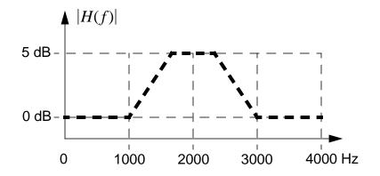
(c) The signal  $s(t) = 10.0 \cos^2(12000\pi t)$  is sampled at 8 kHz using an A/D converter with an anti-aliasing filter that attenuates the analog signal 100 dB at 4 kHz. Compute the output of the system if it is applied to your filter.
