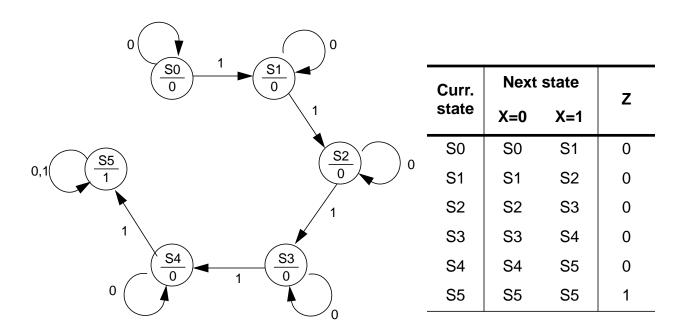
**b)** Use the implication chart method to identify equivalent states. Remove redundant states and draw the minimum state table.
