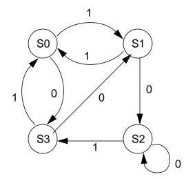
The network described by the adjacent state graph is to be implemented using a 74S163 counter and external logic gates.
