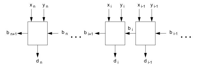
The  $i^{th}$  cell implements  $d_i = x_i - y_i - b_i$  with  $b_{i+1}$  as the borrow to be propagated to the next cell.
