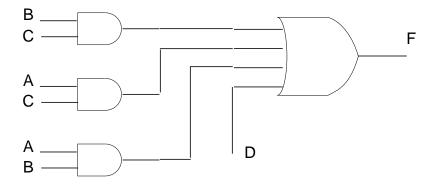
Now we convert this to a NAND-only network by changing all gates to NAND, and complementing the variables connected directly to the output gate. The resulting network is
