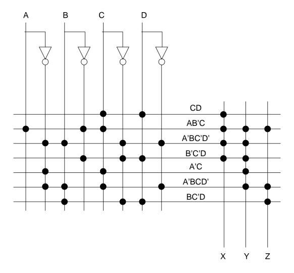
Note that we split the A'BD' term for Y and used the A'BC'D' and A'BCD' terms used for X and Z instead to generate it.
