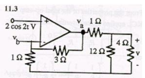
Since the op-amp attempts to maintain zero voltage difference between the inverting and the non-inverting terminal,
