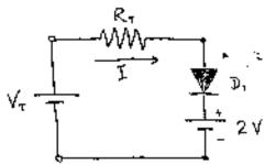
The Thèvenin equivalent resistance is  $R_{\tau} = 500 \parallel 1000 = \frac{1000}{3} \text{ sc}$
