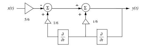
(a) Find the transfer function of this system using Laplace transforms.
