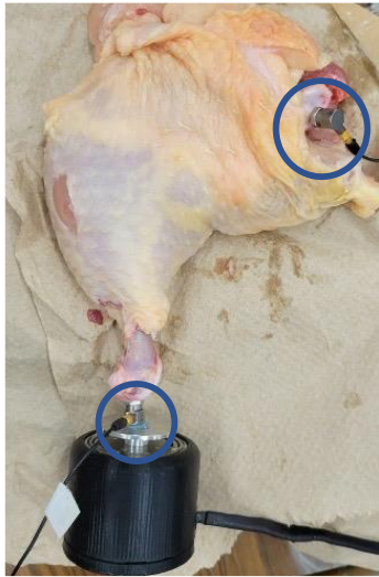
Figure 1. The completely intact knee joint setup. One sensor was positioned at the femoral head, and the other at the distal end of the tibia.
