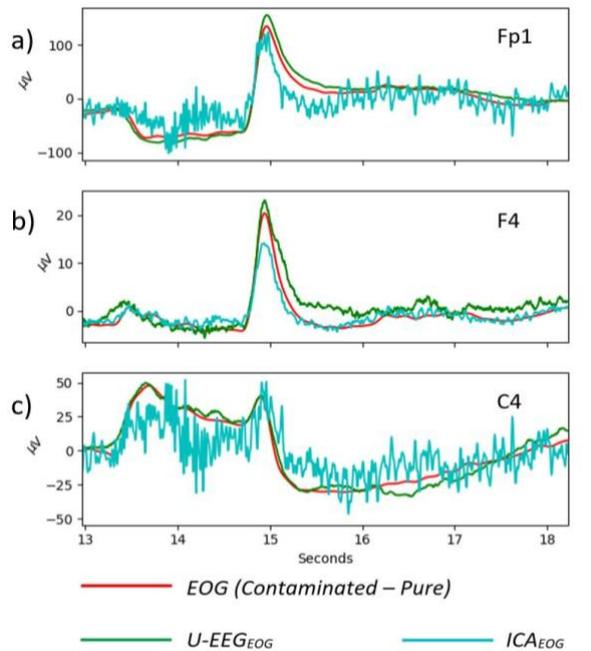
Figure 3. Comparison of U-EEG and ICA EEG artifact detection on test subject 4, depicting randomly selected electrodes Fp1, F4, and C4 within a randomly selected time window (13-18 s). Traces from Fp1, F4, and C4 (a-c) show the EOG artifact (*Contaminated – Pure*) and the EOG estimates *U-EEG<sub>EOG</sub>* and *ICA<sub>EOG</sub>*. For display purposes, the y-axis scale showing EEG amplitude ( $\mu\text{V}$ ) is not constant across subplots.
