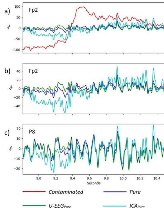
Figure 2. Comparison of U-EEG and ICA filtered EEG signal on test subject 0, depicting randomly selected electrodes Fp2 and P8 within a randomly selected time window (9-10.5 s). Subplot (a) shows *Contaminated*, *Pure*, and the filtered outputs at Fp2. Traces from Fp2 (b) and P8 (c) show the noise-free signal (*Pure*) and estimates  $U\text{-EEG}_{Pure}$  and  $ICA_{Pure}$ . For display purposes, the y-axis scale showing EEG amplitude ( $\mu\text{V}$ ) is not constant across subplots.
