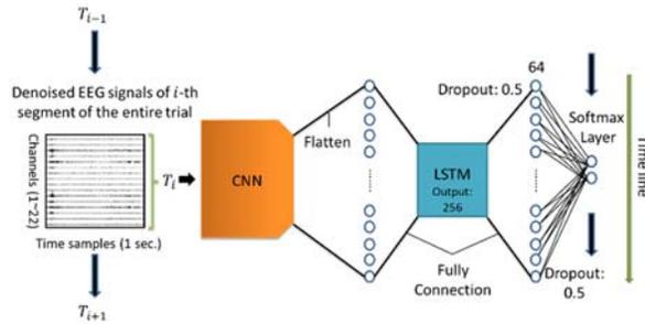
Figure 5: General structure of our model for data processing in one time-step.
