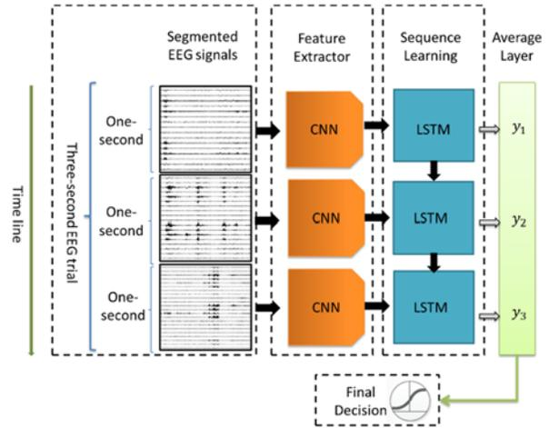
Figure 4: Framework of proposed method: The sequential data consists of three sub segments of the three-second EEG trial. Each time step data is EEG signals of the one-second segment. The CNN extracts features from the preprocessed EEG signals, and the following LSTM network learns the long-term dependencies in the sequential data. An epoch's label is obtained by taking the average on outputs of the Softmax layers of all time-steps.
