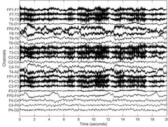
Figure 1: EEG signal contaminated with EMG artifacts. This artifact can be seen with high frequency ( $>30$  Hz) activity in some channels such as FP1-F7 (patient ID 00000177).
