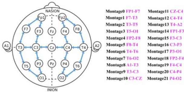
Figure 3: TCP or double banana montage which is used in clinical seizure detection.
