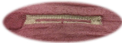
Fig. 1. We use a knit-fabric antenna (made with conductive thread) and an RFID tag as a strain gauge sensor.
