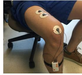
Fig. 3. Placement of EMG Sensor Electrodes
