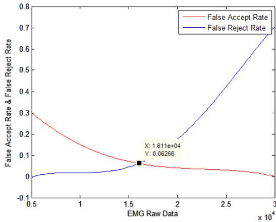
Fig. 5. EMG Threshold Settings
