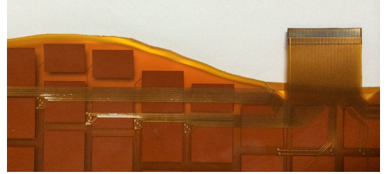
Fig. 3. The real pressure sensor array design and wire connection.
